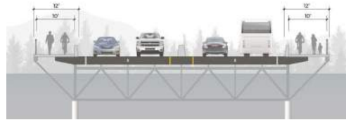
Recommended Alternative: Alternative 2 - 10' Clear Width Walkways on Both Sides of the Bridge
